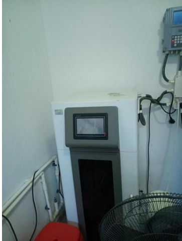
SVL-COD (Cr) 化学需氧量在线监测装置
